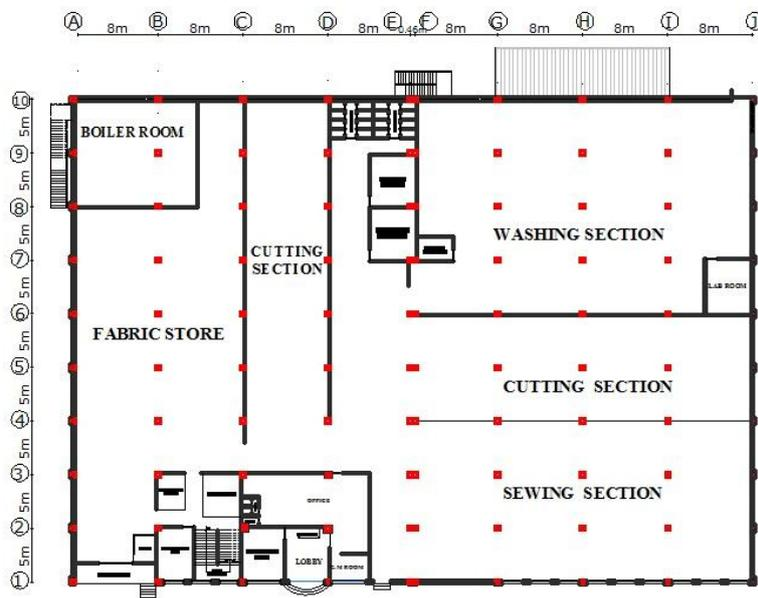
Figure 2: Typical layout plan of 3 storied industrial building
