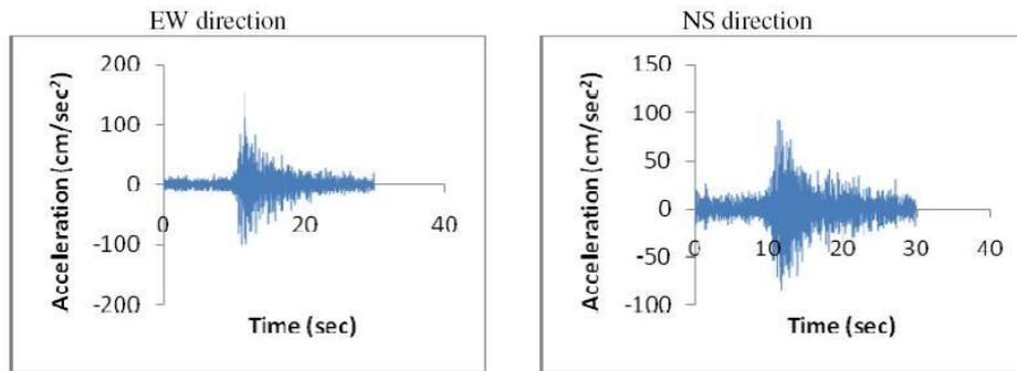
Figure 6: Modified Earthquake Time History of Dhaka
