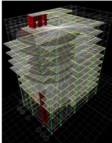
Figure 1: 3D Model of the Concrete Structures
