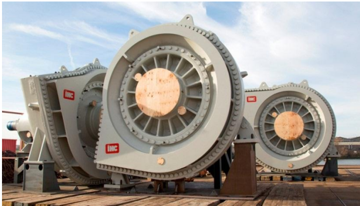
Figure 7: cutter special pump provides a good balance between efficiency, sphere passage
