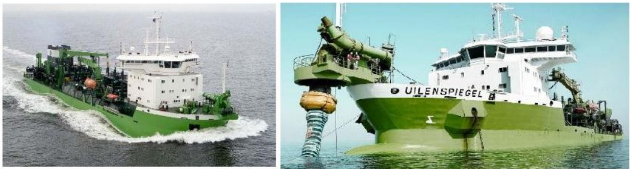
Figure 6: Left, the traditional hull shape; right, the improved bulbous hull resulting reduced fuel Consumption
